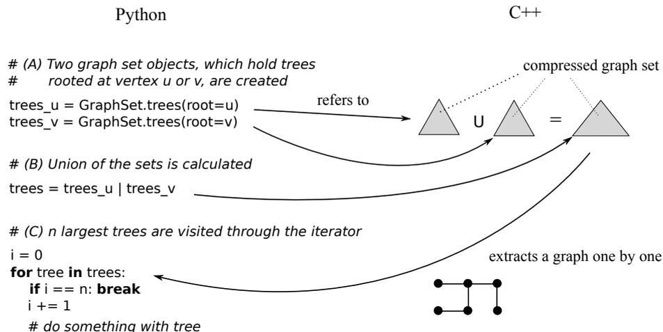
Figure 1: Graphillion’s overview with a code example. The compressed graph set objects are maintained in the C++ world, while only minimum necessary objects are exposed to the Python world to reduce the overhead.
