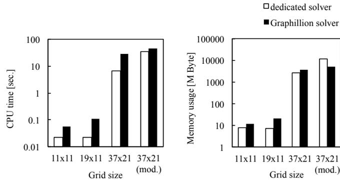
Figure 7: CPU time and memory usage of the dedicated solver and the Graphillion solver on Slitherlink problems.
