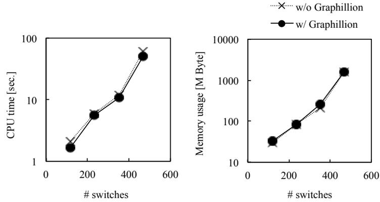
Figure 10: CPU time and memory usage of power network optimizers with and without Graphillion.
