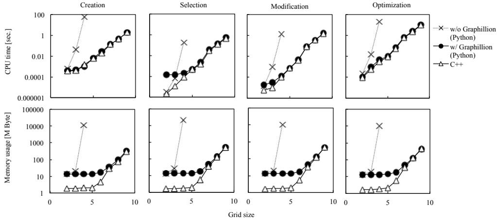
Figure 4: CPU time and memory usage for the basic operations with and without Graphillion. The operations are executed over trees rooted at a corner on a grid graph. The grid size on the horizontal axis indicates  $N$  of the  $N \times N$  grid.
