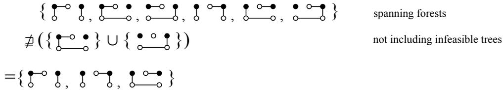
Figure 9: An example of optimization algorithms for power networks in Fig. 8; feasible solutions are obtained as the spanning forests with no infeasible trees, and then the optimal one is searched for (not shown in the figure).
