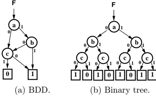
Figure 1: BDD and binary tree:  $F = (a \wedge b) \vee \bar{c}$ .
